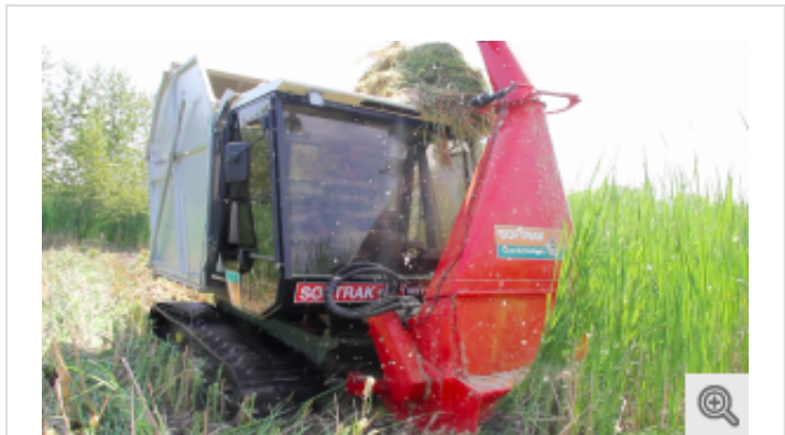
A wetland plant harvester removes non-native cattails from Cheboygan Marsh. The project, based at the U-M Biological Station, is the first large-scale effort to restore a Great Lakes wetland by harvesting invasive plants. Image credit: Levi Stroud
