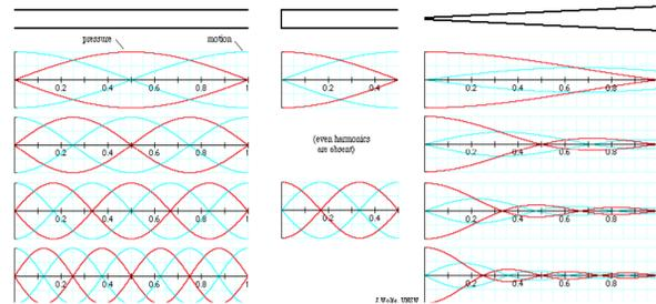
Figure 1: Standing Wave Boundary Conditions [2]
